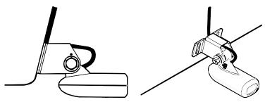
Route cable over bolt and through bracket. Side view (left) and shown from above (right).
